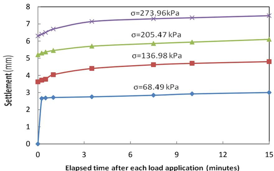
Figure (2): Time-Settlement Curves for Point (1)
