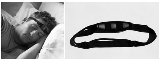
Fig.13 Three dry silver-coated cloth sensors are included in the headband, which is roughly the size of a tennis headband [57].
