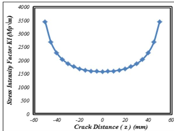
Figure 10: Variation of KI with crack distance (z).
