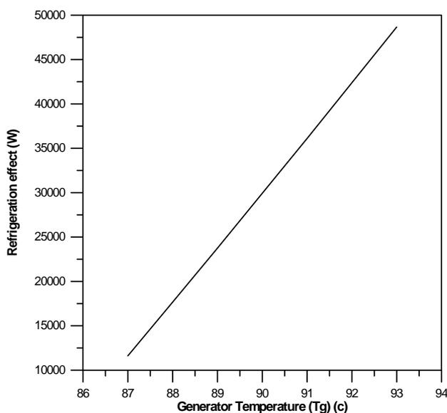
Figure (4). Variation of cooling effect ( $Q_{ev}$ ) with generator temperature .
