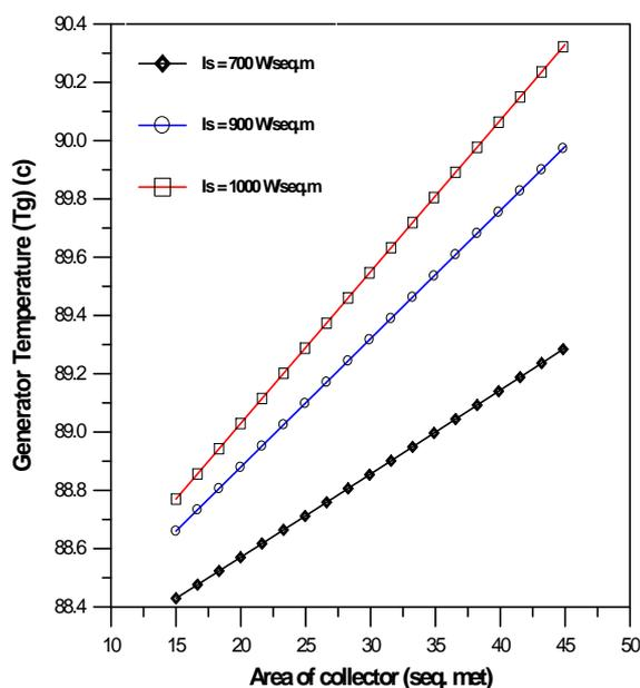
Figure(2). Variation of generator temperature with area of collector for  $T_{amb} = 45 \text{ C}^{\circ}$ .
