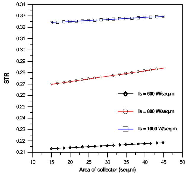
Figure (11). Variation of solar thermal ratio with collector area at  $T_{amb}=45^\circ \text{ C}$ .
