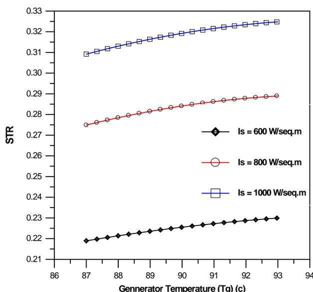
Figure (7). Variation of solar thermal ratio with generator temperature at  $T_{amb} = 45 \text{ }^\circ\text{C}$
