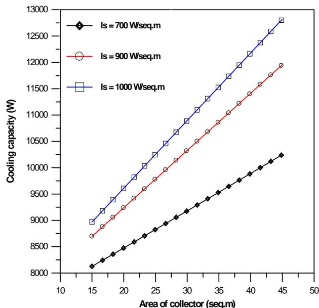
Figure (9). Variation of cooling effect with collector area at  $T_{amb} = 45^{\circ}C$ .
